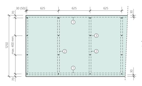
Horizontal profile (axial distance max 1250 mm)
