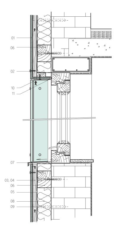
Detail of jamb and window head with sheet metal cladding of opening, CETRIS<sup>®</sup> boards on wooden grid, VARIO system Horizontal and vertical section
