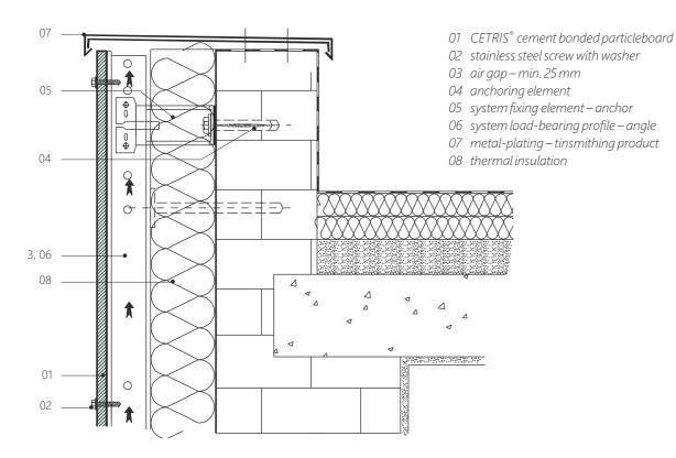
Detail of bottom ending with overlap. CETRIS<sup>®</sup> board on system profiles, VARIO system Vertical section
