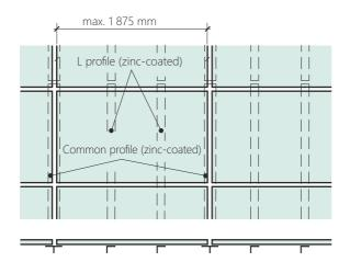
Correct assembly of L profiles at the vertical joint
