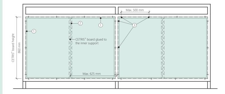
When using a CETRIS<sup>®</sup> board of thickness 10 mm, the maximum possible spacing of the inner vertical reinforcements is 420 mm. A suitable type of the peripheral lath is the F profile PROAL 74008.
