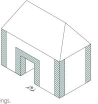
Exposed positions on building edges, openings, passages and thoroughfares in the buildings.
